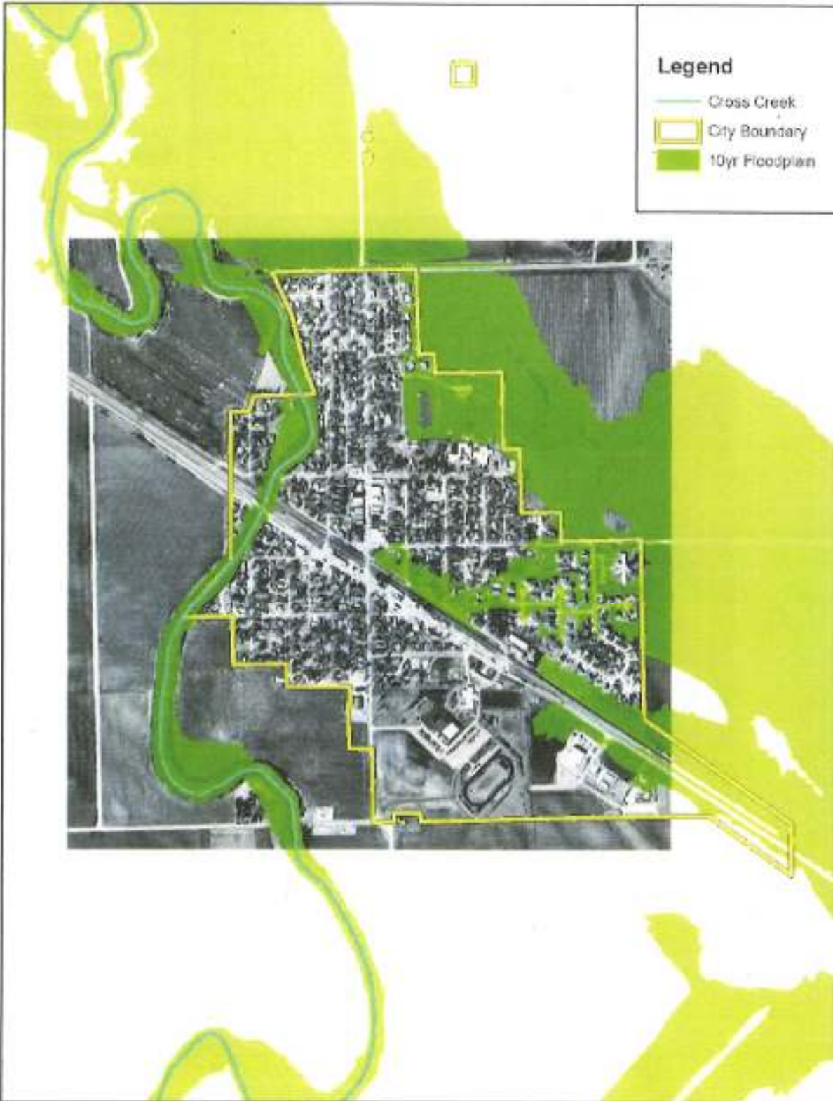
FIGURE 2: EXTENT OF 10% ACE FLOODING WITHOUT BRIDGES FROM CDM 2010 REPORT
